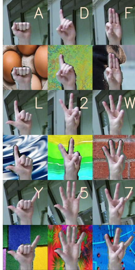
Figure 6: Samples of hand gesture images with original (labeled images) and substituted backgrounds (below originals). Note the remnants of the original backgrounds. This phenomenon is due to dilation of the binary masks. While it could be avoided by using techniques like chroma key, we do not intend to use a uniform background, to avoid bringing any extra apparatus in operation. In the experimental results (Sect. 5.4), we show that despite these remnants, gesture detection is highly accurate.
