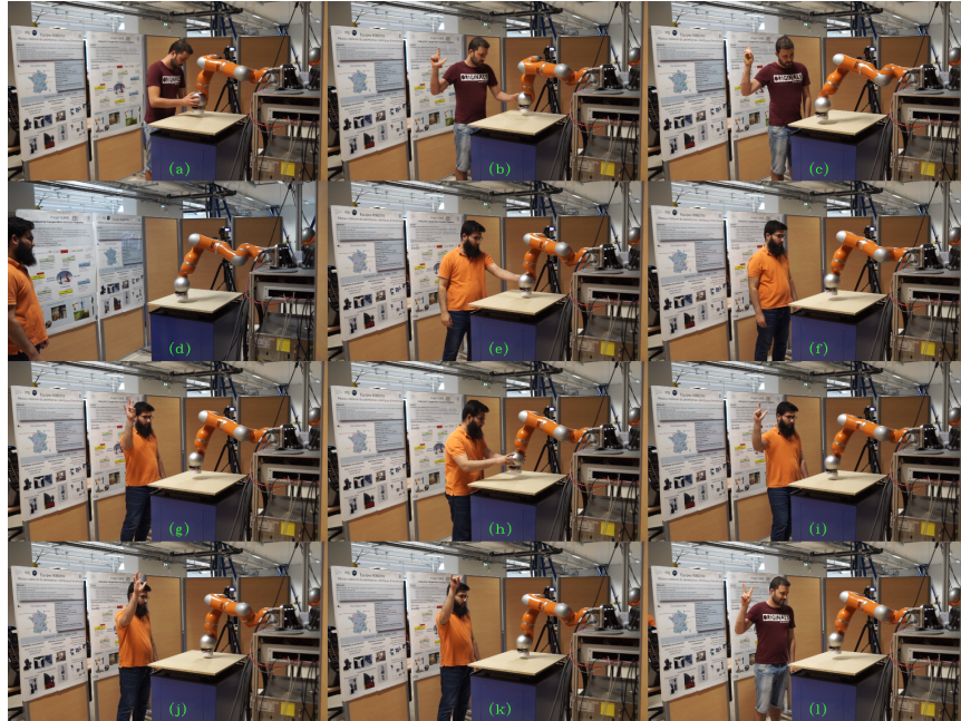
Figure 13: Screenshots from the robotic experiment by operators Op1 and Op2 (a) Op1 manually guiding the robot to a waypoint in the workspace. (b) Op1 records the way-points using Record gesture. (c) Op1 replay the taught waypoints by Replay gesture. (d) Op2 stands far from the robot so it moves with full speed. (e) Op2 stops the robot by applying external force (or accidental touch). (f) Op2 stands near the robot, so it moves slowly ensuring operator's safety. (g) Op2 gives Reteach command to the robot. (h) Op2 sets the new waypoints manually. (i) Op2 gives Record command. (j) Op2 stops the robot by Stop gesture. (k) Op2 resumes the robot operation by Resume gesture. (l) Op1 ends the robot operation by giving End command.
