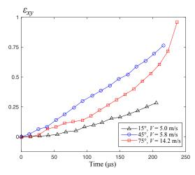
Fig. 17 Normalized shear strain  $\varepsilon_{xy}$  as a function of time for 15°, 45° and 75° loading conditions
