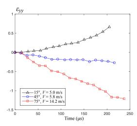
Fig. 18 Normalized normal strain  $\varepsilon_{yy}$  as a function of time for 15°, 45° and 75° loading conditions
