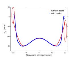
Fig. 9 Numerical simulation : normal stress  $\sigma_{yy}$  as a function of distance to joint centre, with and without beaks
