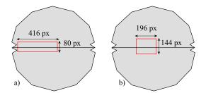
Fig. 11 a) Imaging area for 15° and 45° loading conditions. b) Imaging area for the 75° loading condition
