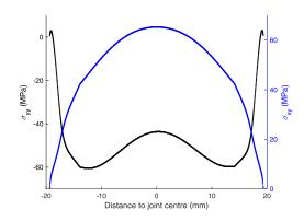
Fig. 7 Numerical simulation: normal stress  $\sigma_{yy}$  (*black line*) and shear stress  $\sigma_{xy}$  (*blue line*) versus the distance to the joint centre for the 45° loading condition
