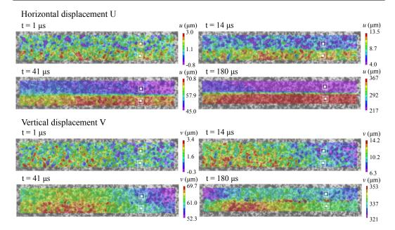
**Fig. 16** Horizontal (top) and vertical (bottom) displacement field measured by DIC for the 45° loading condition at v = 5.8 m/s at different times: 1 µs, 14 µs, 41 µs and 180 µs
