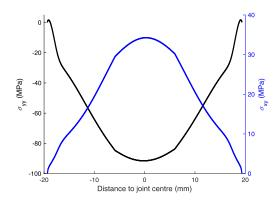
Fig. 8 Numerical simulation: normal stress  $\sigma_{yy}$  (*black line*) and shear stress  $\sigma_{xy}$  (*blue line*) versus the distance to the joint centre for the 75° loading condition
