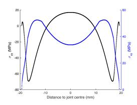
Fig. 6 Numerical simulation: normal stress  $\sigma_{yy}$  (black line) and shear stress  $\sigma_{xy}$  (blue line) versus the distance to the joint centre for the 15° loading condition
