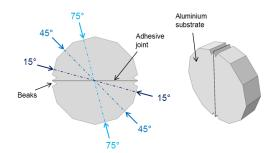
Fig. 2 Schematic view of the DODECA specimen
