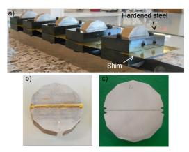
Fig. 4 a) Specimens before curing and bonding devices. b) Specimen just after curing. c) Final specimen ready to be tested
