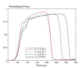
Fig. 13 Normalized force as a function of time for the 45° loading condition
