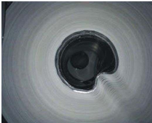
(a) Local buckling
