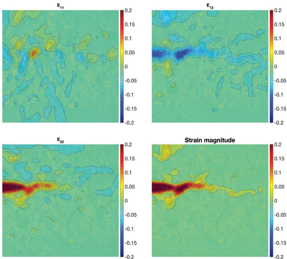
**Figure 6.** Strain field measured by [Figure 5](#) image correlation.
