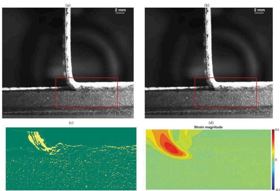
**Figure 4.** Example of digital image correlation on large-frame images: (a) reference image, (b) deformed image, (c) grey-level residual map after digital correlation, and (d) resulting strain magnitude.
