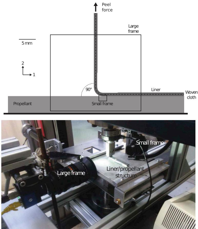
**Figure 1.** Experimental setup.
