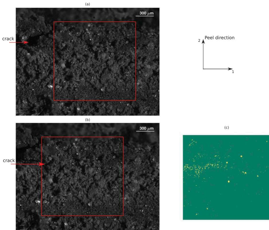
**Figure 5.** Example of digital image correlation on small-frame images: (a) reference image (the crack has not entered the red box yet), (b) deformed image (the crack has entered the box), and (c) grey-level residual map after image correlation.
