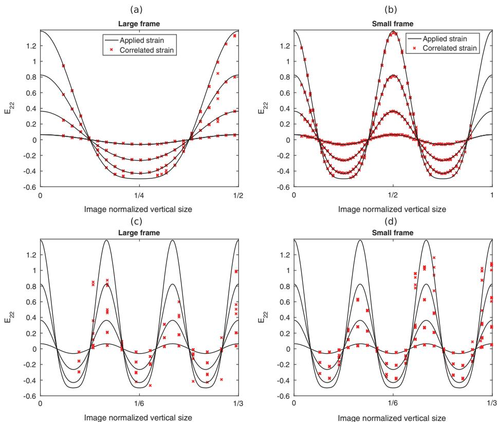
**Figure 2.** Speckle performances: comparison between artificially applied sinusoidal unidirectional pixel displacements and image correlation estimates for a large period of half the image size with (a) large-frame image (spray painting) and (b) small-frame image (natural texture) and for a small period of one-tenth of the image size with (c) large frame and (d) small frame.
