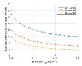
Fig. 3: Power efficiency for fixed user/BS ratio
