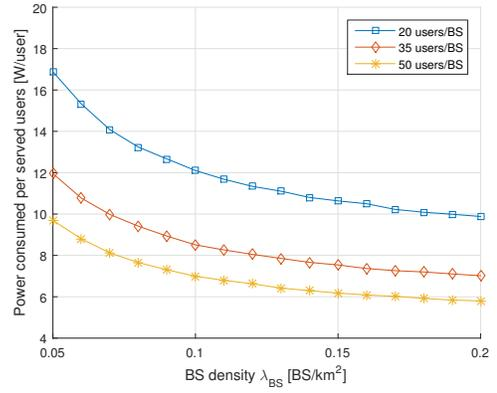
Fig. 3: Power efficiency for fixed user/BS ratio
