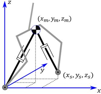
Fig. 1: A simplified model of a 3D biped robot. Each leg is massless and has variable length. At the contact point, the stance leg rotates passively around axes  $x$  and  $y$ , the rotation around axis  $z$  is not considered since this rotation is usually inhibited by friction in normal biped locomotion. The swing leg has a fully actuated spherical joint with respect to the concentrated mass of the hip.
