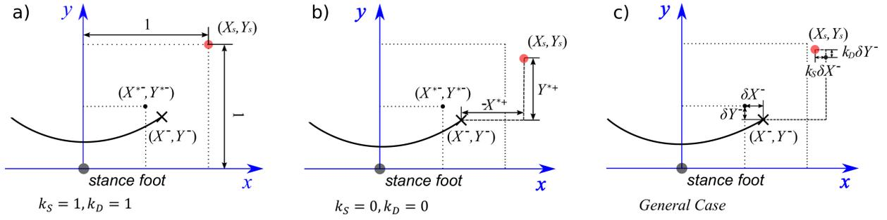
Fig. 3: Influence of  $k_S$  and  $k_D$  on the foot locations. a) Step length and width are fixed; b) The initial CoM position error is nullified; c) The general case. The black and the red dots represent respectively the stance feet during the current and the next steps. The curved line represents the CoM trajectory, and the cross the CoM position at the end of the current step.
