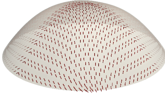
Figure 7: Example one, shape and material optimization: optimal shape and orthotropy direction field.
