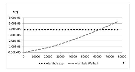
**Figure 7.** Comparison of failure rate  $\lambda(t)$  for Prj3.
