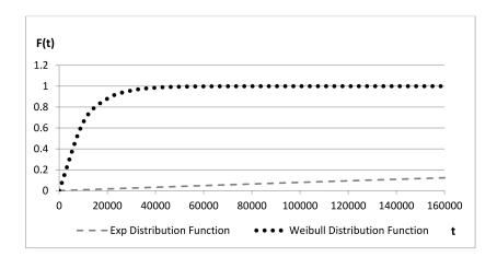
**Figure 9.** Comparison of cumulative distribution functions F(t) for Prj2.
