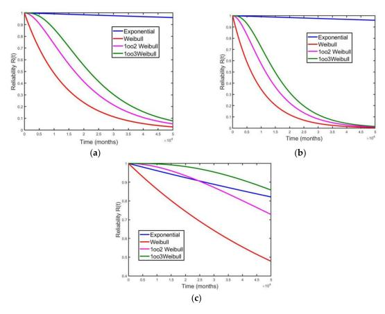
**Figure 11.** Reliability functions with redundancies k-out-of-n. Solutions for (**a**) project Prj1; (**b**) project Prj2; and (**c**) project Prj3.
