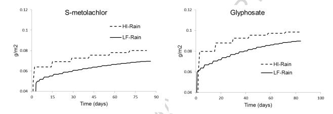
**Figure 7.** Cumulative pesticide wash-off from mulch obtained from the model simulations. Symbols HI-R and LF-R represent heavy and infrequent and light and frequent rain regimes, respectively.
