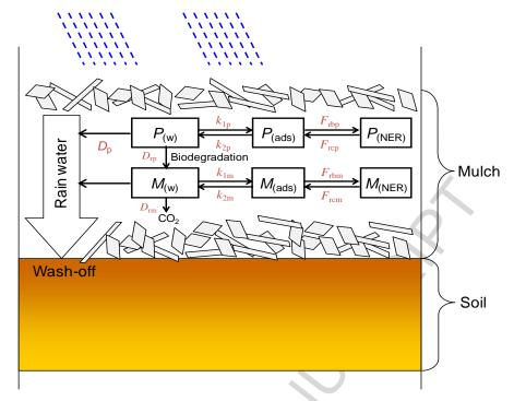
**Figure 1.** Schematic diagram of the pesticide module in mulch. Pesticide compartments of soluble (w), adsorbed (ads) and non-extractable residues (NER) of the parent molecule (P) and metabolite (M) are represented. The soluble compartment diffuses in rain water and can leach into soil below the mulch.
