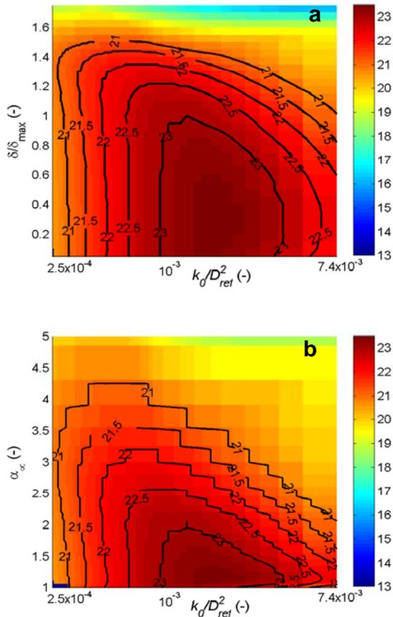
Figure 8. Insertion Loss  $IL_{1000\text{Hz}}$  (dB) response surfaces corresponding to various membrane closure rates  $\delta/\delta_{\text{max}}$  (a) or tortuosities  $\alpha_{\infty}$  (b) and dimensionless static permeabilities  $k_0/D_{\text{ref}}^2$  at porosity 0.95.
