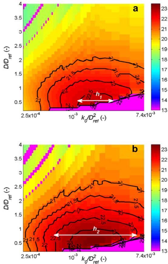
Figure 7. Insertion Loss  $IL_{1000\text{Hz}}$  (dB) response surfaces corresponding to various dimensionless cell sizes  $D/D_{ref}$  and dimensionless static permeabilities  $k_0/D_{ref}^2$  at porosities 0.90 (a) and 0.95 (b).
