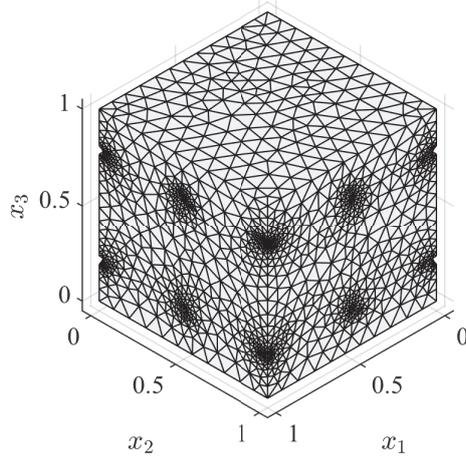
FIG. 9. Meshed view of the equivalent microstructure.
