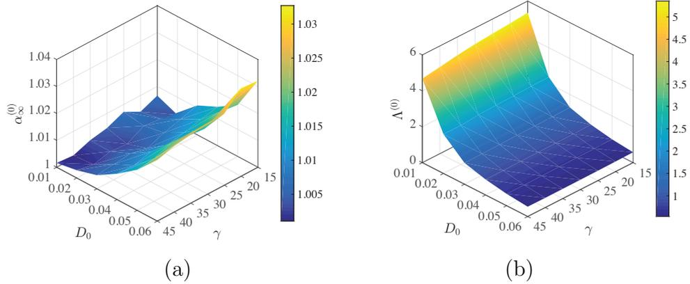
FIG. 11. This figure shows the graphs of (a) the high-frequency tortuosity  $\alpha_\infty^{(0)}$  and (b) the viscous characteristic length  $\Lambda^{(0)}$  associated with  $\Omega_0$ , as a function of  $D_0$  [-] and  $\gamma$  [°].
