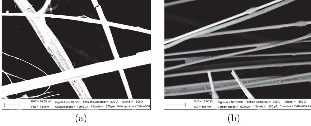
FIG. 2. Examples of micrographs. The scale bar in the SEM images is  $5 \times m_D$ , where  $m_D$  is the mean diameter of the analyzed fibers (see Eq. (28) for a detailed definition of  $m_D$ ). (a) Horizontal plane. Sample size is equal to  $48.4m_D \times 32.5m_D$ . (b) Vertical plane. Sample size is equal to  $41.5m_D \times 27.8m_D$ .
