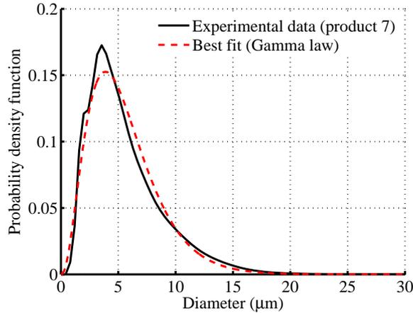
FIG. 3. (Color online) The estimated probability density function of fiber diameter is shown for product 7.
