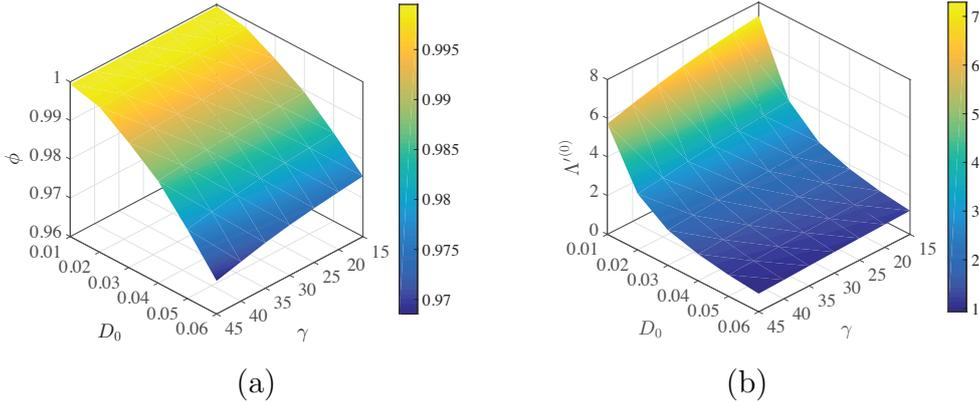
FIG. 8. (Color online) This figure shows the graphs of (a) the macroscopic porosity  $\phi$  and (b) the thermal characteristic length  $\Lambda^{(0)}$  associated with  $\Omega_0$ , as a function of  $D_0$  [-] and  $\gamma$  [°].
