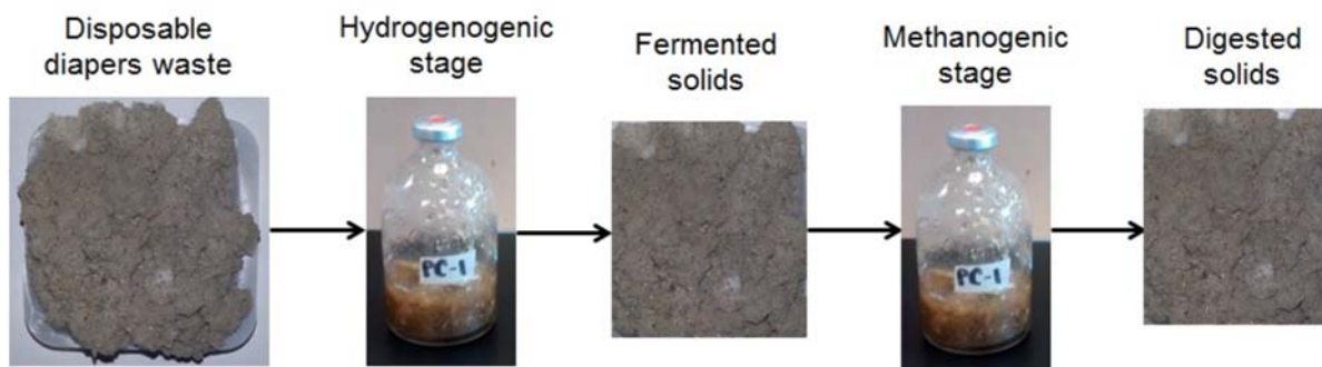
FIGURE 7. Two-stage experimental set-up for solid substrate fermentation.
