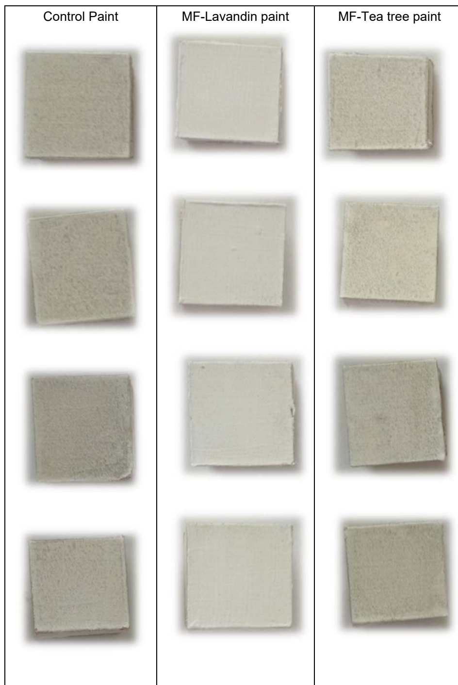
FIGURE 4. Antifungal assay on paint film containing MF-EO exposed to Aspergillus sp. after 4 weeks (quadruplicate)
