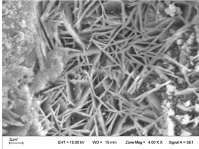
FIGURE 7: Micrograph of MIC phenomenon metabolites
