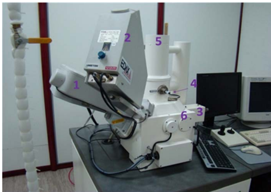
FIGURE 3: Scanning Electron Microscope. 1) WDS spectrometer, 2) EDS spectrometer, 3) Backscattered electron detector, 4) Secondary electron detector, 5) Electron gun, and 6) Chamber
