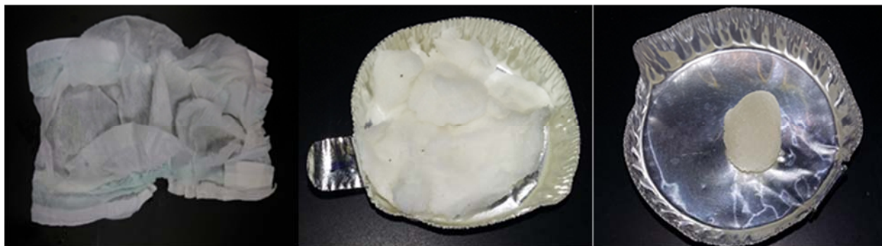
FIGURE 2. Disposable diaper separated by components (plastic, pulp cellulose and Ca-P)
