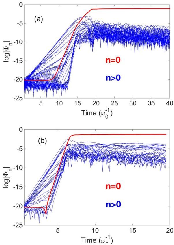
FIG. 4. Temporal evolution of the potential amplitude, for  $n = 0$  to  $n = 30$ . The mode  $n = 0$  is highlighted in red. Case (a):  $G_Z = -20$  where TIMs are dominant, case (b):  $G_Z = +20$  where TEMs are dominant.
