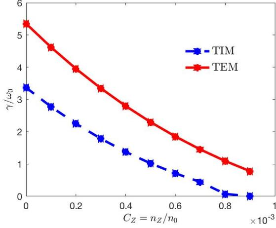
FIG. 1. Growth rate of the fastest growing mode of TIMs and TEMs as a function of the tungsten impurity density  $\mathcal{C}_z$ . Only  $n_Z$  is changed,  $n_0$  is the electron density and remains constant. The blue dots correspond to TIM growth rates, the red dots correspond to TEM growth rates.
