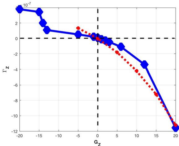
FIG. 5. Averaged impurity flux  $\Gamma_z$  as a function of  $G_Z$ . The dots correspond to simulation points (in blue). In red (dotted line) is shown the particle flux estimated from the mixing length estimate ( $\Gamma_z \propto -\gamma G_Z$ ) and using the linear growth rates of the TEM instability as a function of  $G_Z$  (see Fig. 3).
