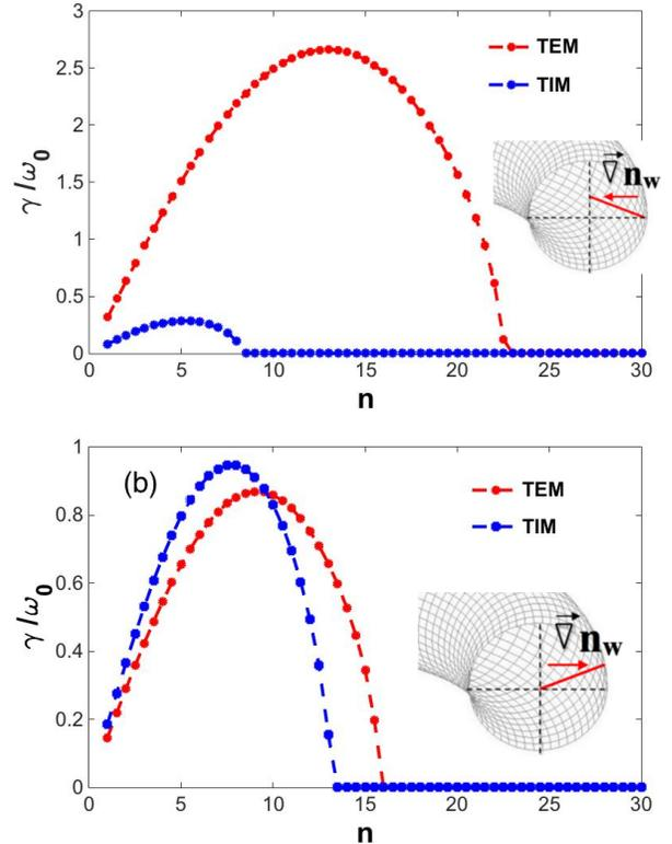
FIG. 2. Growth rate of TEMs and TIMs as a function of mode number. Case (a):  $G_Z = +20$ , case (b):  $G_Z = -20$ . The blue dashed curve corresponds to the growth rate of the TIM modes, the red solid curve corresponds to the growth rate of the TEM modes. For clarity, negative growth rates have been set to zero. The poloidal cross section sketches display the shape of the impurity profile for negative and positive  $G_Z$ .
