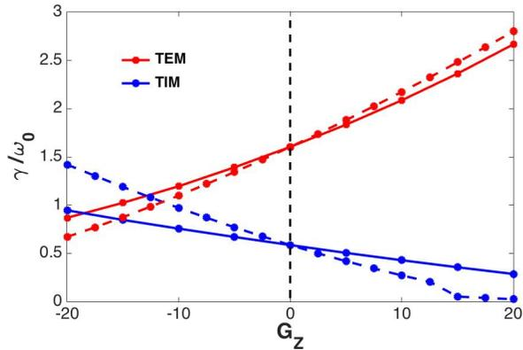
FIG. 3. Linear growth rate of the fastest growing mode as a function of the impurity gradient length  $G_Z$ . The blue solid (dotted) curve corresponds to TIM growth rates, the red solid (dotted) curve corresponds to TEM growth rates, keeping  $\kappa_{n_i}$  ( $\kappa_{n_e}$ ) constant.
