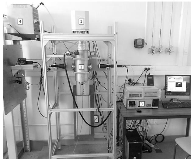
Fig. 2. Sorption isotherm device with: 1-Magnetic suspension balance; 2-Heating jacket enclosing the measuring chamber; 3-Humidity generator; 4-Shiller for temperature control.
