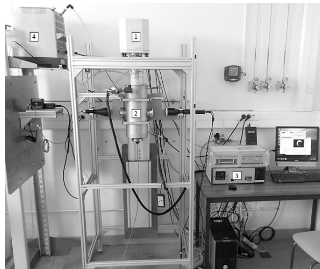
Fig. 2. Sorption isotherm device with: 1-Magnetic suspension balance; 2-Heating jacket enclosing the measuring chamber; 3-Humidity generator; 4-Shiller for temperature control.
