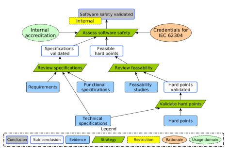
**Fig. 2.** JPD illustrates the result of kick-off of a new project. Requirements must lead to functional and technical specifications that must be reviewed to be validated. Due to this refinement, technical hard points are found and feasibility studies need to prove that they can be overcome.
