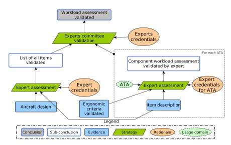
Fig. 6. Justification Pattern-Diagram at stage 3
