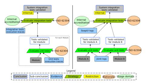
**Fig. 1.** Justification Pattern-Diagram (JPD) on right and the associated Justification Diagram (JD) on left in the context of automated tests execution.
