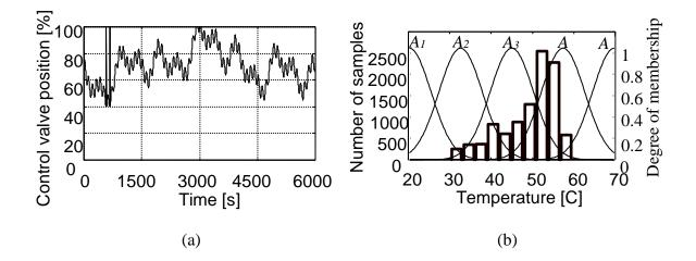
Figure 3 Characteristics of the signals used for identification: (a) time sequence of the input signal; (b) histogram of the output signal superimposed with the membership functions.
