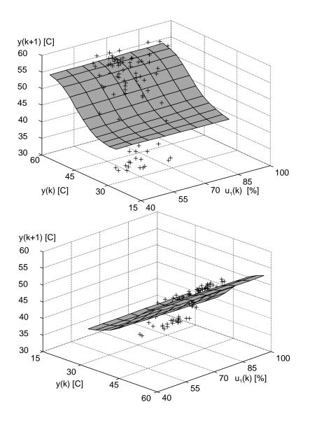
Figure 5 The surface of the identified fuzzy model (considering only the valve position as an input) and the experimentally measured points seen from two angles. The measured points are distributed in space around the surface. The dispersion of the measured points is due to the inputs not considered in the model.
