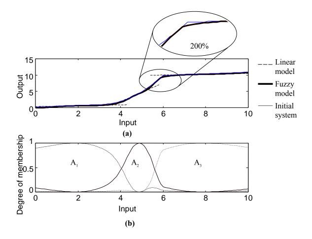
Figure 2 Identifying a Sugeno-type fuzzy model using membership functions
