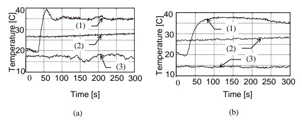
Figure 6The controlled outlet temperature of a fan-coil when the set point is<br/>changed from 20°C to 35°C: a) Sugeno-fuzzy controller; b) PID with anti-<br/>wind up. The three temperatures represent: (1) the fan-coil outlet<br/>temperature; (2) the indoor air temperature of the test cell; (3) the outdoor<br/>air temperature.
