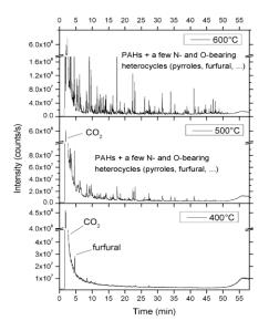
Figure 2 - Chromatograms obtained after a 400°C (bottom), 500°C (middle) and 600°C (top) pyrolyses of 20mg of JSC Mars-1.
