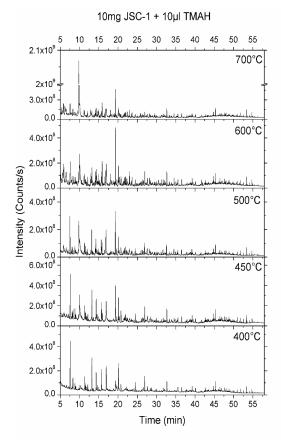
Figure 4 – Chromatograms obtained after thermochemolyses of 10mg of JSC Mars-1 between 400°C and 700°C.
