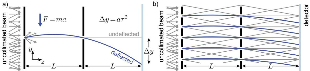
Figure 3 – a) Two slits separated by a distance  $L$  restrict the path of a beam to a specific trajectory. b) Replacing the slits by two gratings increases the flux of particles reaching the detector. A third grating (not shown here) located at the level of the detector allows one to take advantage of the moiré effect to reveal macroscopic fringes.
