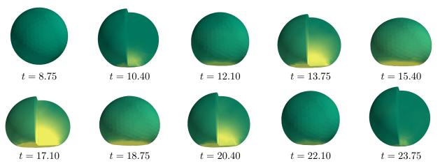
Figure 19: First bounce of the sphere. Von Mises stress distribution. One view over two is a sectional one.
