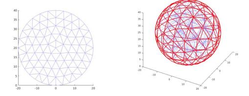
Figure 17:  $P_2$  meshes used for the ball and the sphere.
