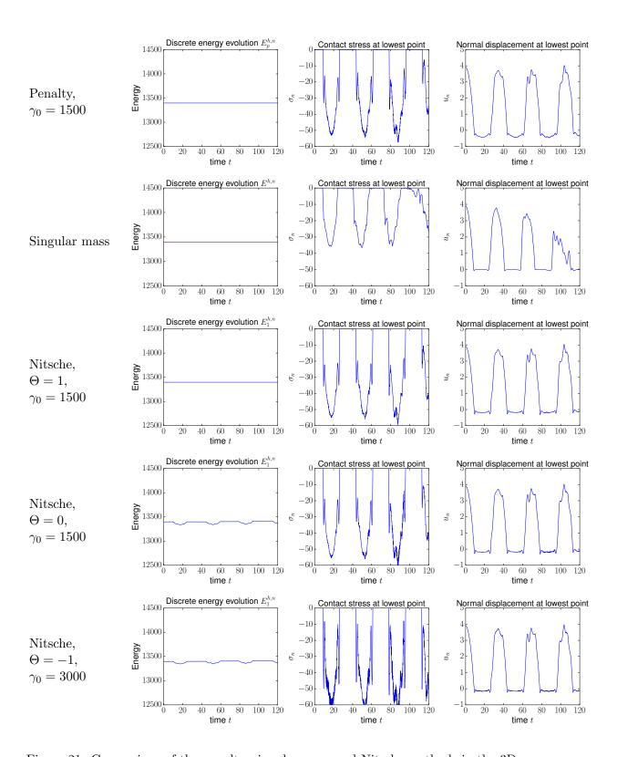
Figure 21: Comparison of the penalty, singular mass and Nitsche methods in the 3D case. For space semi-discretization, Lagrange isoparametric finite elements of order k=2 have been
