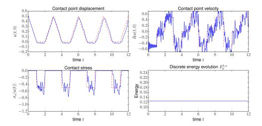
Figure 13: Multiple impacts of an elastic bar. Penalty method for h = 1/20,  $\tau = 0.01$ ,  $\gamma_0 = 1$  and  $P_1$  Lagrange finite elements.
