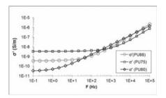
Figure 1. Real electric conductivity of 3 PUs at room temperature.
