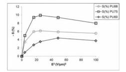
Figure 3. Evolution of the strain amplitude in function of the square of the electric field amplitude.
