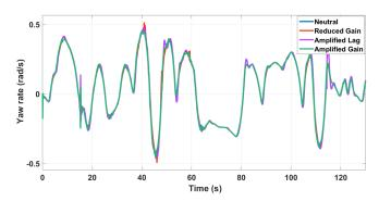
Fig. 2. Yaw rate responses in case of reference tuning.
