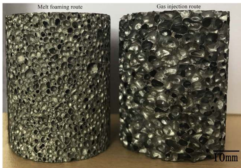
Fig. 3. The two aluminium foam specimens for true density experiments.
