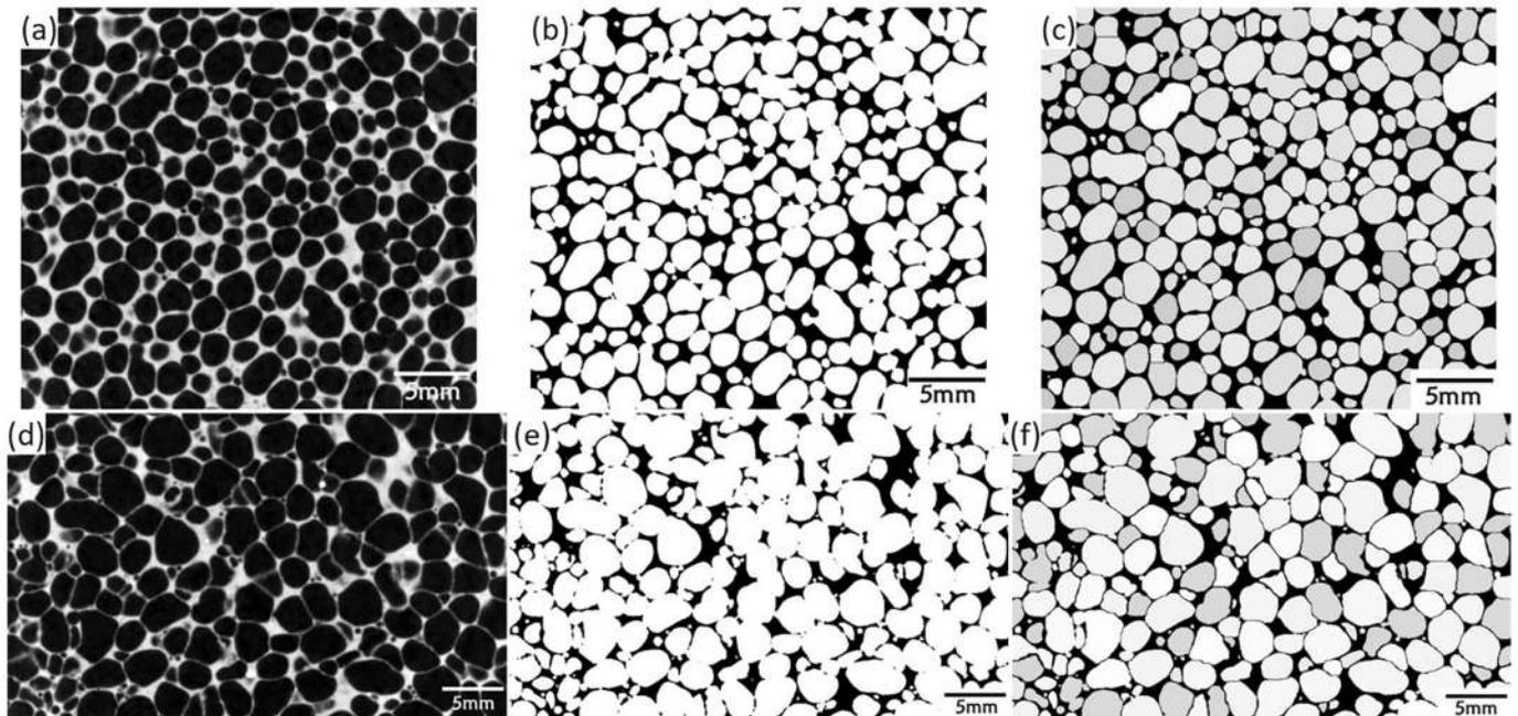
Fig. 9. Cell split processes of (a)–(c) the MF74 (the calculated average cell size with this method is 1.89 mm, and the standard deviation  $s$  is 0.462 mm) and (d)–(f) the GI80dyn ( $\bar{d}$  is 2.62 mm, and  $s$  is 0.696 mm). (a) and (d) are original scanned 2D images, (b) and (e) are images after binarization, (c) and (f) are images after using “3D watershed split”.
