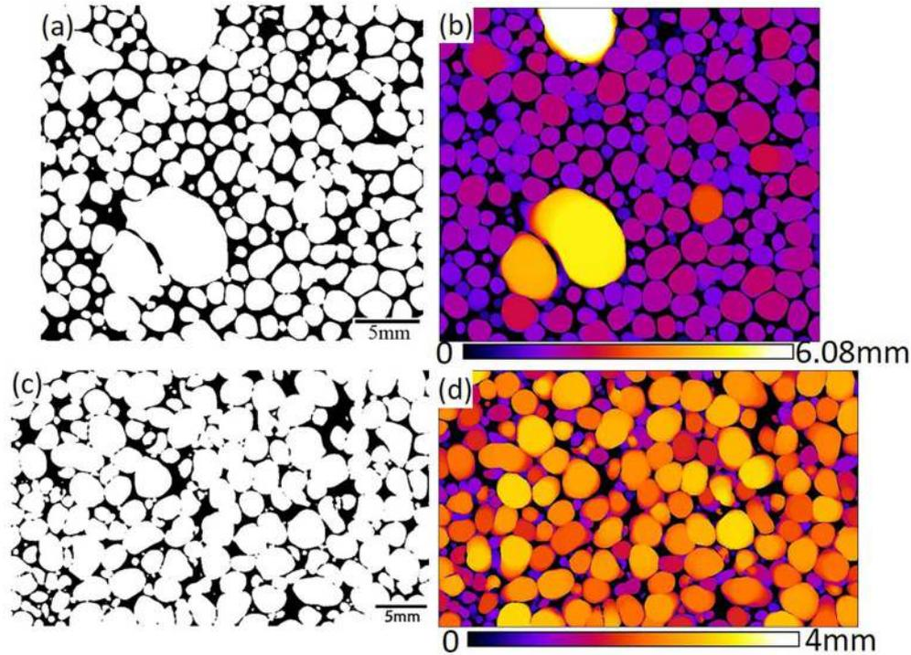
Fig. 8. (a) Binarized image and (b) the image after calculating with “Local Thickness” of the MF74 (the calculated average cell size  $\bar{d}$  with this method is 1.73 mm, and the standard deviation  $s$  is 0.606 mm), (c) binarized image and (d) the image after calculating with “Local Thickness” of the GI80dyn ( $\bar{d}$  is 2.08 mm, and  $s$  is 0.619 mm).
