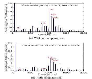
Fig. 9. Stator current spectrum with and without compensation
