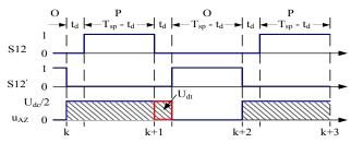
(b) Dead-time effect of switching states O and P with  $i_{ra} < 0$
