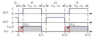
(a) Dead-time effect of switching states O and P with  $i_{ra} > 0$
