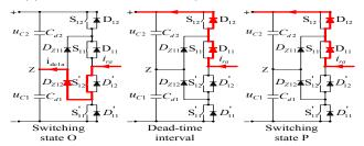
(b) Commutation from switching state O to P with  $i_{ra} < 0$
