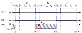
(d) Dead-time effect of switching states N and O with  $i_{ra} < 0$
