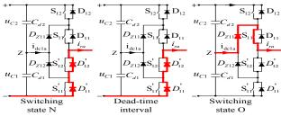
(c) Commutation from switching state N to O with  $i_{ra} > 0$
