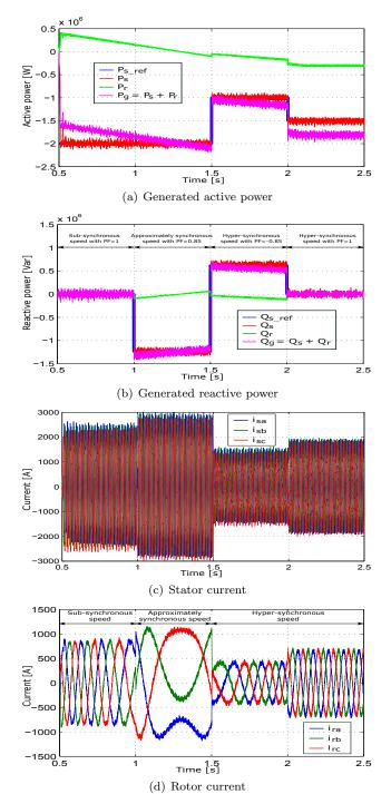
Fig. 8. The dynamic response of the power and current with rotor speed variation
