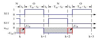
(c) Dead-time effect of switching states N and O with  $i_{ra} > 0$
