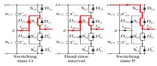
(a) Commutation from switching state O to P with  $i_{ra} > 0$
