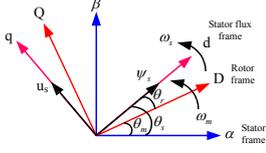
Fig. 3. Vector representation in different reference frame
