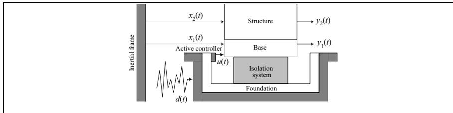
Figure 1. *Building structure with hybrid control system.*
