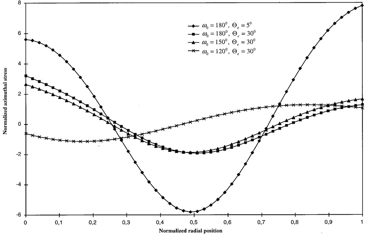
Fig. 3 Azimuthal stresses distribution inside the wall with fibers (stresses normalized by  $\sigma_{r\theta}(r_e)$ ,  $\mu=0.166$  Mpa,  $E_f = 10$  Mpa,  $p_i=0.0133$  Mpa,  $\tau_f=2$  mm,  $\tau_e=3$  mm)
