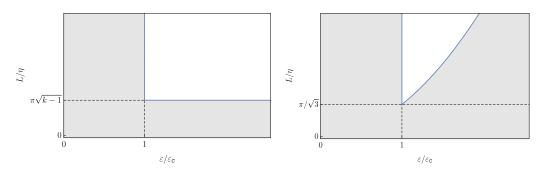
Figure 4: Conditions for the local uniqueness of the homogenous response as a function of the loading ( $\varepsilon/\varepsilon_c$ ) and the normalized bar length ( $L/\eta$ ). Light gray indicates regions where the homogeneous response is locally unique, hence stable. Left: (LS) model; right: (NS) model.
