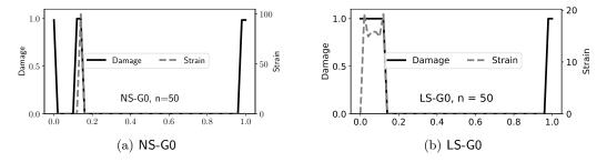
Figure 13: Strain-Gradient models SG0: the results of the numerical simulations show uncontrolled localization of the damage and strain fields and are extremely sensitive to the mesh, imperfections and solver parameters. The figures show a snapshot of the damage and strain field at t = 2.0 for  $\eta/L = 0.2$  and n = 50 elements.
