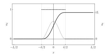
Figure 9: Minimising sequence (74) for the SG0 model with E(1) = G(1) = 0. Black solid line: displacement  $u_{\delta}$ ; dashed line: damage  $\alpha_{\delta}$ ; gray solid line: strain  $\varepsilon_{\delta}$ .
