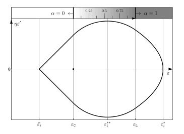
Figure 7: Plot of the localised solution curve  $\eta \varepsilon'_i = \pm \sqrt{F_i(\varepsilon_i)}$  in the  $(\varepsilon, \eta \varepsilon')$  plane when  $\varepsilon^*_i > \varepsilon_{\rm L}$ . The color bar at the top of the plot gives the value of the damage field  $\alpha_i$  calculated as a function of  $\varepsilon_i$  using (14). The qualitative properties of this curve are given in Proposition 5.1.
