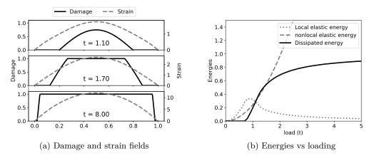
Figure 11: Strain-Gradient model LS-G1: numerical results for the traction test. The simulation is without imperfection for  $\eta/L = 0.2$  and n = 300 elements.
