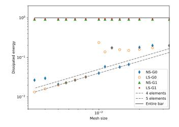
Figure 12: Strain-Gradient models: dissipated energies vs. mesh size at the end of the loading process. Markers are data from numerical simulations. The dashed and continuous lines serve as reference giving the dissipated energies corresponding to the full damage of few elements or of the whole bar.
