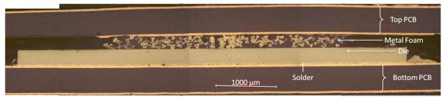
Fig. 2. Metalurgical cut of an embedded diode. The die and the foam are, respectively, 254 and 220  $\mu$ m-thick.
