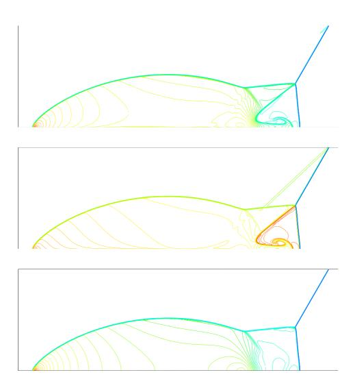
Fig. 4.12. Double Mach reflection – From top to bottom: density, internal energy and pressure at t=0.2, obtained with  $h=2.5\ 10^{-3}$ ,  $\delta t=2.5\ 10^{-5}$  and  $\nu=0.01$ . The variation ranges of the unknowns are  $\rho\in[1.4,\ 22.35],\ e\in[1.786,\ 63.53]$  and  $p\in[1,\ 536]$ . A right part of the domain, where the solution is constant, is not drawn.
