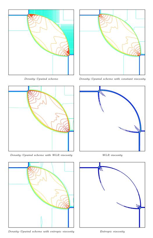
Fig. 4.9. A two-dimensional Riemann problem: Configuration 4 in [30] – h=1/400 and  $\delta t=h/10$  – Results at t=0.3.
