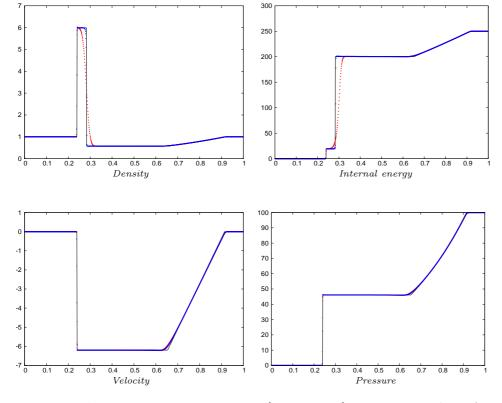
Fig. 4.4. A 1D Riemann problem: Test 4 of [39, Chapter 4] – h = 0.001 and  $\delta t = h/30$  – Results at t = 0.035. The upwind and MUSCL solutions are drawn in red and blue respectively, the analytical solution corresponds to the black line.
