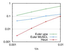
Fig. 4.2. A 2D Regular problem with constant pressure and velocity –  $L^1$  errors on the density at t=0.8 obtained with three different schemes: first-order time discretization (Euler scheme) and first order upwind convection scheme, first-order time discretization and MUSCL convection scheme and Heun time discretization and MUSCL convection scheme. The space step is h=3.2/n with  $n=100,\ 200,\ 400,\ 800$  and the time step is  $\delta t=h/8$ .
