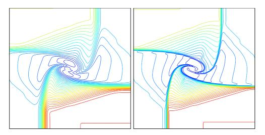
Fig. 4.8. A two-dimensional Riemann problem: Configuration 6 in [30] – Comparison of the upwind (left) and MUSCL (right) schemes – h = 1/400 and  $\delta t = h/10$  – Density at t = 0.3.
