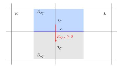
Fig. 3.1. Notations for the construction of the corrective term  $S_{K,1}$ , in the MAC case, for a dual face lying on the primal cells boundaries.  $\epsilon$ : considered dual edge.  $D_{\sigma_{\epsilon}^{u}}$ : upstream dual cell.  $D_{\sigma^{d}}$ : downstream dual cell. K, L: upstream cells.
