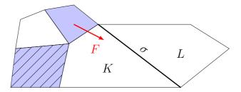
Fig. 3.2. Limiting process – For  $\sigma = K|L$  and with a constant advection field  $\mathbf{F}$ , the possible calidates for the upstream cell  $M_{\sigma}$  are coloured in blue; the unique opposite cell is hatched.
