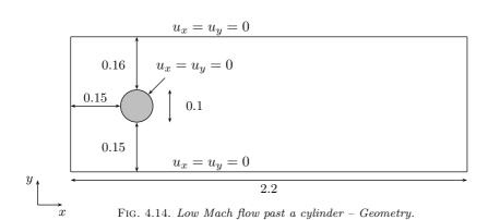
**4.6.** A Mach=10 flow past a cylinder. The last test case is a compressible version of a benchmark originally developed for incompressible Navier-Stokes solvers [36]. The geometry of the problem is described in Figure 4.14. The fluid enters the domain on the left boundary with a constant velocity:
