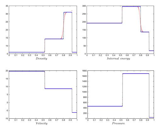
Fig. 4.5. A 1D Riemann problem: Test 5 of [39, Chapter 4] – h=0.001 and  $\delta t=h/90$  – Results at t=0.035. The upwind and MUSCL (with artificial viscosity) solutions are drawn in red and blue respectively, the analytical solution corresponds to the black line.
