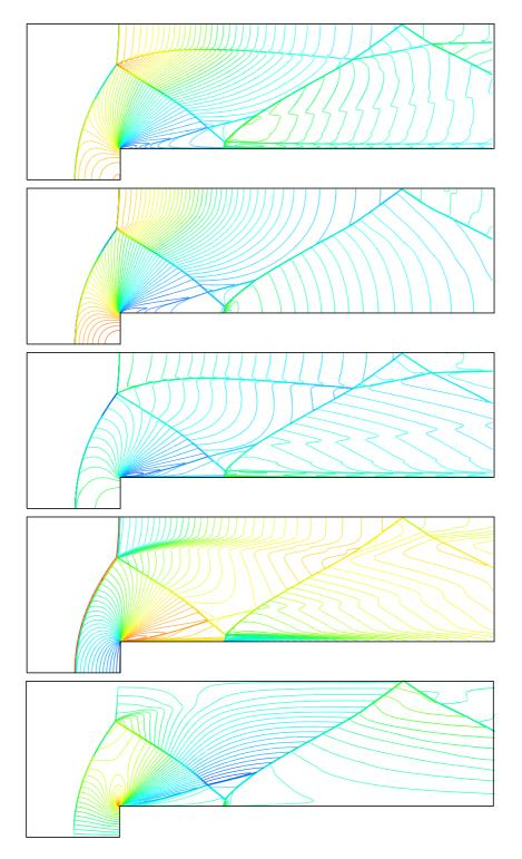
FIG. 4.10. Mach 3 step – From top to bottom: density, pressure, internal energy, first and second component of the velocity at t=4, obtained with  $h=2.5\times 10^{-3}$ ,  $\delta t=10^{-3}$  and  $\nu=10^{-3}$ . The variation intervals of the unknowns are  $\rho\in[0.235,\ 6.4],\ p\in[0.216,\ 12.04],\ \mathcal{H}\in[2.46,8.11],\ u_1\in[0.,\ 3.046],\ and\ u_2\in[-0.92,\ 1.82].$
