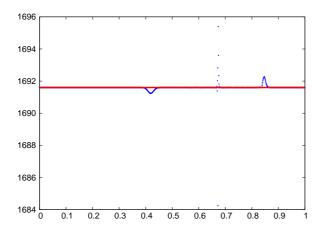
Fig. 4.3. A 1D Riemann problem: single contact discontinuity – h = 0.001 and  $\delta t = h/40$  – Pressure at t = 0.02. Results obtained with a correlated (resp. non-correlated) face approximation for  $\rho$  and e are drawn in red (resp. in blue). The analytical solution is the same as the discrete solution obtained with the correlated approximation (non-visible black line).
