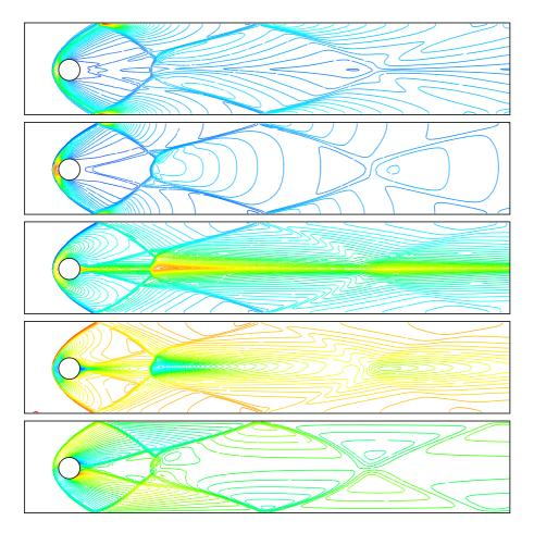
Fig. 4.16. Mach=10 flow past a cylinder – From top to bottom: density, pressure, internal energy, x-component of velocity and y-component of velocity at t=5. The variation ranges of the unknowns are  $\rho \in [0.804,\ 12.23],\ p \in [0.002,\ 1.219],\ e \in [0.178,\ 0.536],\ u_1 \in [-0.11,\ 1],\ and\ the value\ u_1=0\ corresponds\ to\ the\ fourth\ iso-line,\ u_2\in [-0.326,\ 0.327].$
