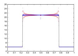
Fig. 4.6. A 1D Riemann problem: the "symetrical double shock" – h = 0.001 and  $\delta t = h/60$  – Density at t = 0.035. Upwind solution without (red) and with (blue) WLR viscosity.
