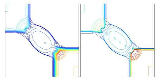
Fig. 4.7. A two-dimensional Riemann problem: Configuration 5 in [30] – Comparison of the upwind (left) and MUSCL (right) schemes – h = 1/400 and  $\delta t = h/10$  – Density at t = 0.23.
