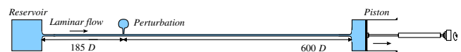
FIG. 1 (color online). Schematic diagram of the pipe flow facility (drawn to scale). The piston moves at a controlled speed and the fluid is pulled through the pipe at constant mass flux. The usable experimental run time is \approx 30 min.
