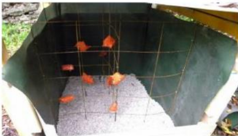
Fig. 4 Implantation of the thermo-buttons protected by tape and a watertight shell
