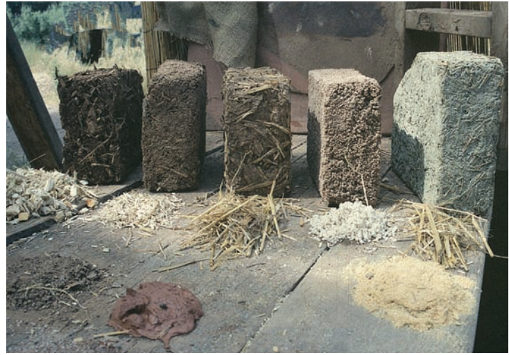
Fig. 5 A range of clay and fiber blocks by Frank Andresen, photo: C. Wanek
