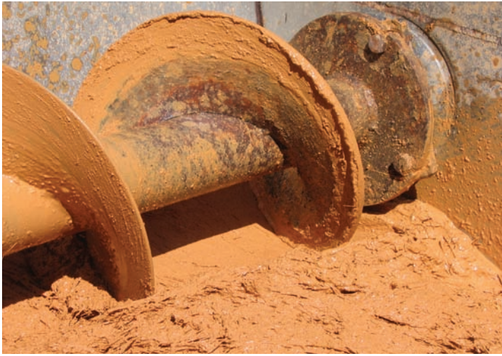
Fig. 4 A silage mixer repurposed to mix earth plaster, photo: J. Kennedy
