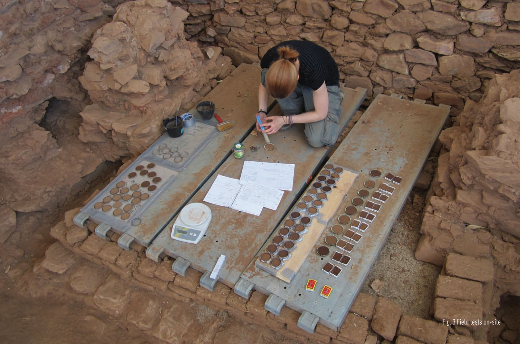
Fig. 4 Hygric dilatation test under high humidity on samples of historic plasters
