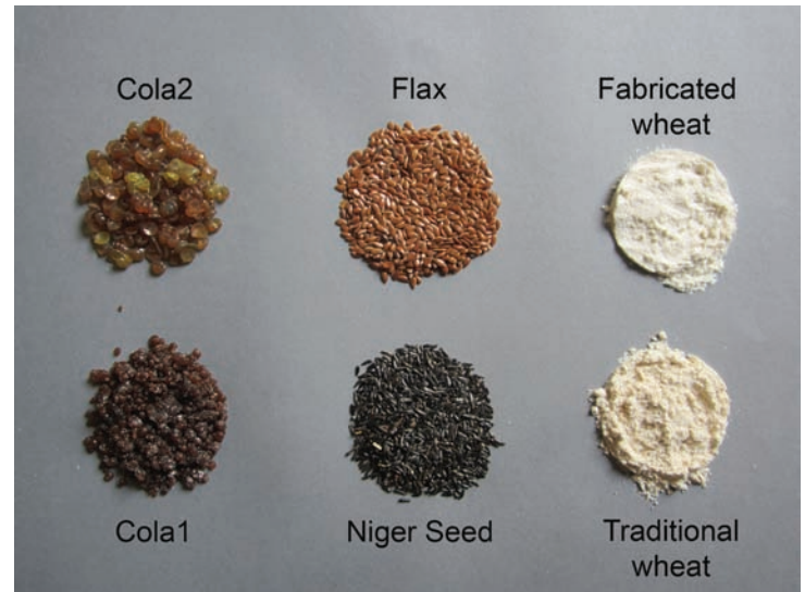
Fig. 2 Ethiopian binders: animal glues (left), seeds (middle) and wheat starch (right)
