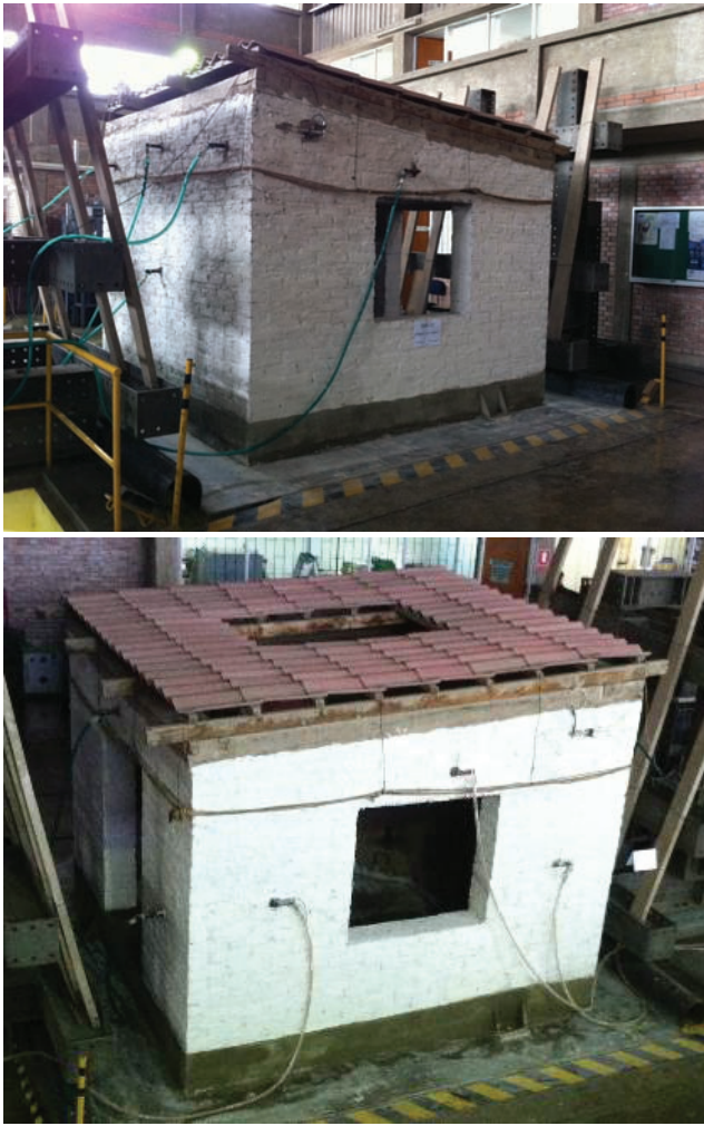
Fig. 1 Adobe model ready to be tested in seismic simulation
