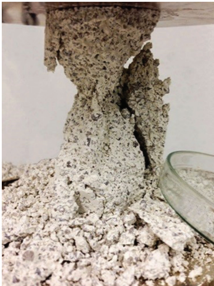
Fig. 1 Sample of "model" earth after mechanical compression test
