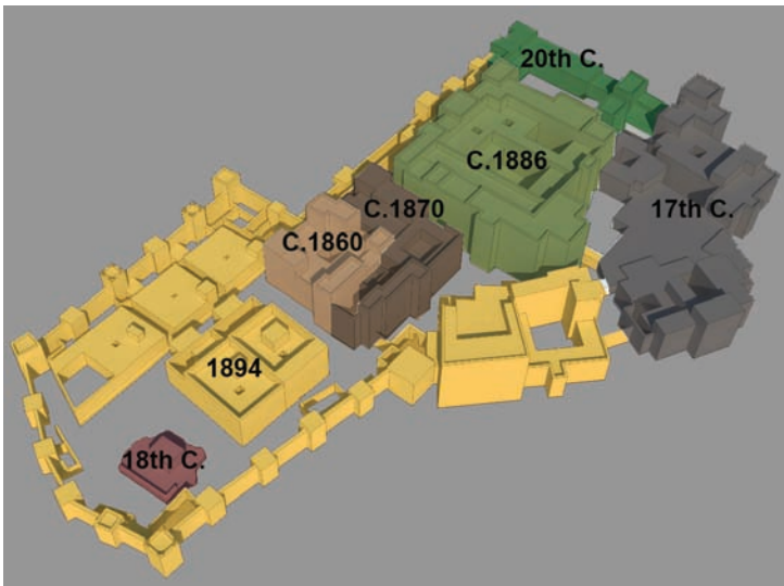
Fig. 5 Model of the kasbah showing construction phases, image: E. Macchioni
