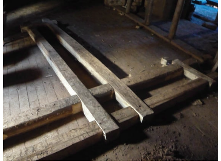
Fig. 3 Corner key assembly in the Laboratory before testing
