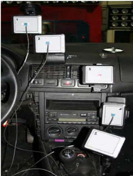
Fig 12: Various types of low-cost customary fitting products for nomadic devices have been tested through crashes
