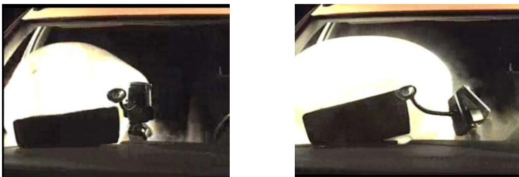
Fig.3: Some pictures of the movie showing the nomadic support smashed by the air bag during the crash test of a vehicle.
