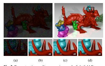
**Fig. 5**: Reconstruction quality comparison on the light field Dragon. Top: (left) 4% sub-sampled view, (right) OFS reconstruction. Bottom: (a) sampled region, (b) RUS, (c) FSR, (d) OFS.
