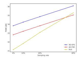
**Fig. 4**: PSNR comparison of 4D-FSR, 4D-OFS methods and RUS [7] for different sampling rates.
