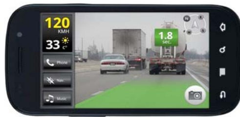
Figure 2: Example of display for smartphone application informing the driver about the safety of the distance with the vehicle in front (on the picture, the color green symbolizes that the distance is safe).
