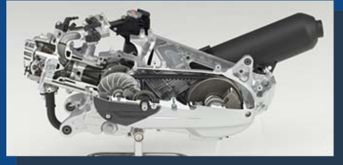
Honda 125cc scooter engine: A 25% more fuel efficient
