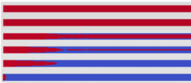
Figure 4 solidification process of liquid aluminium (in red liquid phase, in blue solid phase); a- at start time the tube is completely filled by liquid aluminium, b- the aluminium solidification starts at the tube wall at a distance from the entry, c- the solidified aluminium progress in the radial direction, d- the solidified aluminium close the tube at a section further from the entrance and stops the fluid flow, e- the solidification progress at the entry direction, f- at the end the aluminium is completely solidified
