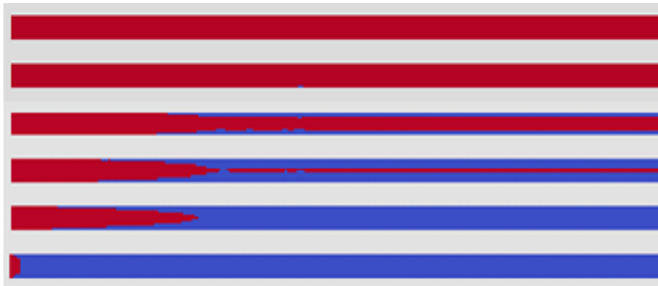
Figure 4 solidification process of liquid aluminium (in red liquid phase, in blue solid phase); a- at start time the tube is completely filled by liquid aluminium, b- the aluminium solidification starts at the tube wall at a distance from the entry, c- the solidified aluminium progress in the radial direction, d- the solidified aluminium close the tube at a section further from the entrance and stops the fluid flow, e- the solidification progress at the entry direction, f- at the end the aluminium is completely solidified
