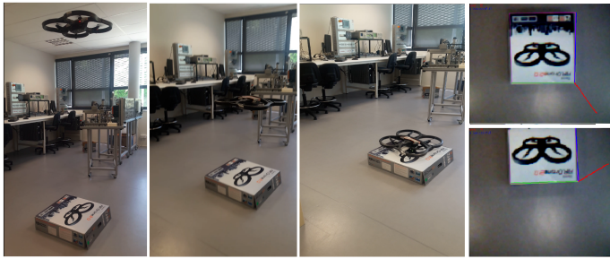
Fig. 7. Visual servoing for homing. On the left: the quadcopter hovering above the landing template and performing a controlled landing. On the right: the view seen from the bottom camera of the quadcopter that shows robustness to occlusion (when the landing object is partially out of the field of view).
