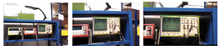
Fig. 6. Localization based on an electrical instrument (oscilloscope): From left to right, images taken from the quadcopter video stream that show how the system can control the quadcopter to obtain a front view of the instrument.
