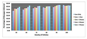
FIGURE I. THE EFFECT OF BUSES ON THE PERCENTAGE OF MESSAGES DELIVERED USING MAXPROP
