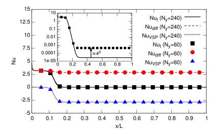
Fig. 13: Streamwise profiles of the total Nusselt number  $Nu_t(x)$ , its diffusive part,  $Nu_{diff}(x)$ , and its part due to VSP,  $Nu_{VSP}(x)$ , for the incompressible slipping flow at  $D_h = 6 \mu m$ ,  $p_{in} = 0.1 \ bar$  and  $p_{out} = 0.09 \ bar$  (see Table 4) and for two uniform Cartesian meshes of size  $N_x \times N_y = 3000 \times 60$  and  $12000 \times 240$ . A zoom on the  $Nu_t$  profiles is included.
