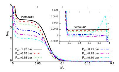
Fig. 15: Streamwise profiles of the total Nusselt number,  $Nu_t(X)$ , for the weakly compressible micro-flows of Table 5, at  $D_h = 6 \ \mu m$ ,  $\Delta p_{ref} = 0.1 \ bar$  and a decreasing average pressure.
