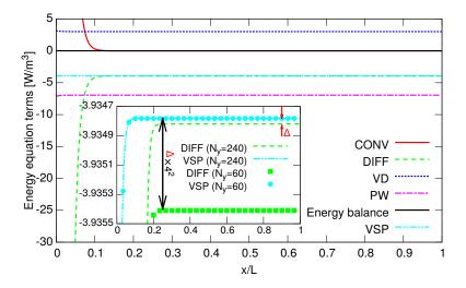
Fig. 12: Streamwise profiles of each term of Eq. (72) and energy balance (CONV + DIFF - PW - VD), for the incompressible slipping flow at  $D_h = 6 \ \mu m$ ,  $p_{in} = 0.1 \ bar$  and  $p_{out} = 0.09 \ bar$  (see Table 4). The zoom shows that  $DIFF \rightarrow VSP$  for two uniform Cartesian meshes of sizes  $N_x \times N_y = 3000 \times 60$  and  $12000 \times 240$ .
