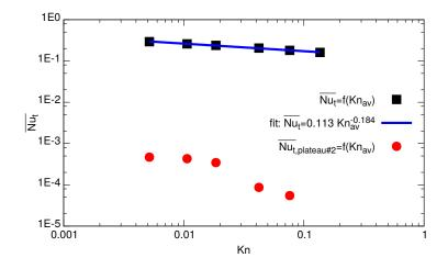
Fig. 16: Integral mean of the total Nusselt number along the whole wall  $(\overline{Nu_t})$  and along the wall part corresponding to the second Nu-plateau  $(\overline{Nu_t}, plateau\#_2)$ , with respect to the average Knudsen number, for the weakly compressible micro-flows of Table 5, at  $D_h = 6 \ \mu m$ ,  $\Delta p_{ref} = 0.1 \ bar$  and a decreasing average pressure.
