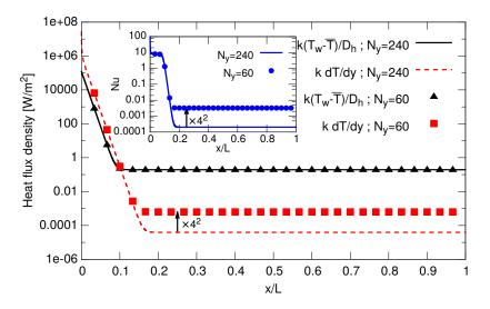
Fig. 11: Streamwise profiles of the Nusselt number Nu (enclosed figure), Nu numerator  $\left(-k \frac{\partial T}{\partial y}\Big|_{w}\right)$  and Nu denominator  $\left(k(T_w - \overline{T})/D_h\right)$ , for the incompressible no slip flow at  $D_h = 6 \ \mu\text{m}$ ,  $p_{in} = 5 \ bar$  and  $p_{out} = 4.99 \ bar$  (Fig. 9) and for two uniform Cartesian meshes of sizes  $N_x \times N_y = 3000 \times 60$  and  $12000 \times 240$ .
