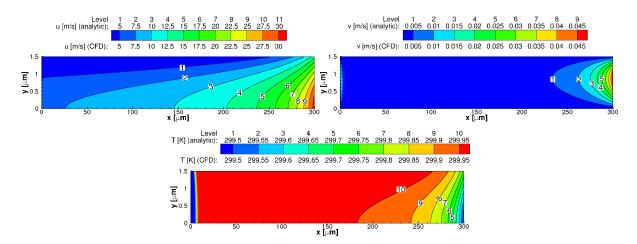
Fig. 3: Comparison of the analytical solution (black isolines) and numerical solution (color fields) for u (top, left), v (top, right) and T (bottom), in case (a). Symmetry is taken into account and a half channel is presented.
