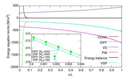
Fig. 14: Streamwise profiles of the thermal energy balance (CONV + DIFF - PW - VD), of its different terms and of the power of the viscous stress at the wall (VSP), for the compressible slipping flow at  $D_h = 6 \ \mu m$ ,  $p_{in} = 0.2 \ bar$ ,  $p_{out} = 0.1 \ bar$  (see Table 5).
