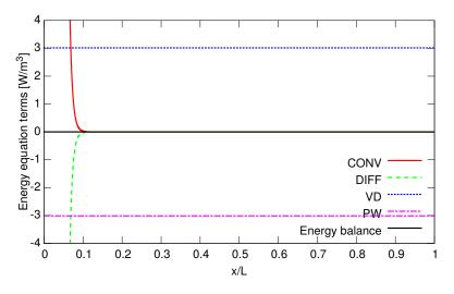
Fig. 10: Streamwise variation of each term of the energy equation integrated on a channel slice (convective (CONV) and diffusive (DIFF) fluxes and pressure work (PW) and viscous dissipation (VD) source terms), and total energy balance (CONV+DIFF-PW-VD), for the no slip incompressible flow at D<sub>h</sub>=6 μm, p<sub>in</sub> = 5 bar, p<sub>out</sub> = 4.99 bar of Fig. 9.
