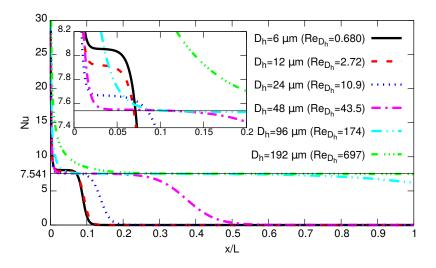
Fig. 9: Profiles of the wall Nusselt number, Nu, with respect to X = x/L, for incompressible no slip flows at various hydraulic diameters and Reynolds numbers ( $p_{in} = 5 \ bar$ ,  $p_{out} =$  $4.99 \ bar$ , L/H = 50). A zoom on the Nu profiles at the channel entrance is included.
