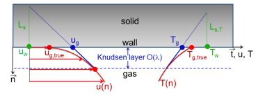
Fig. 1: Schematic representation of the true (in red) and approximated (in blue) velocity and temperature profiles in the Knudsen layer and (in green) of the slip length,  $L_s$ , and temperature jump length,  $L_{s,T}$ .
