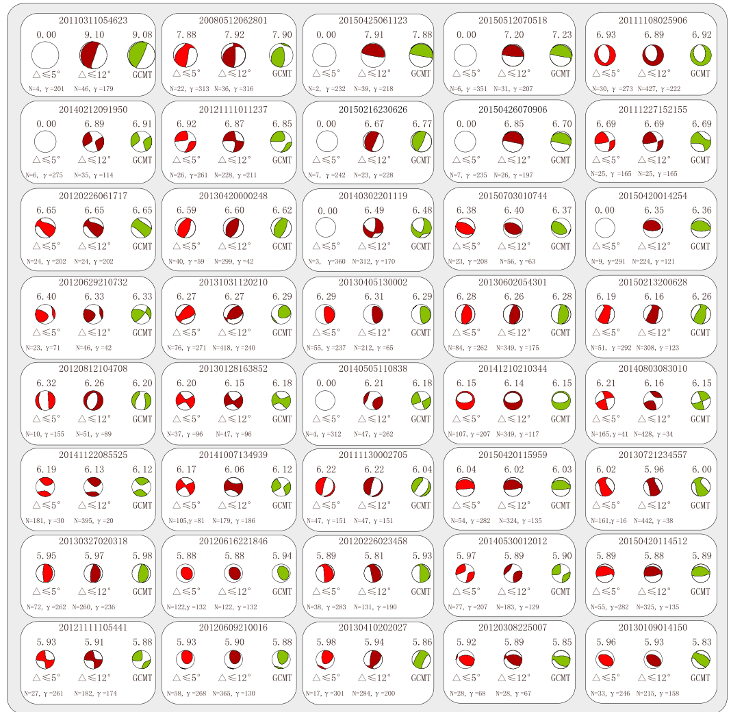
Figure 3. W-phase moment tensor solutions for M_w \geq 5.8 in China and neighboring area from November 2011 to November 2015 along with the 2011 M_w = 9.1 Tohoku and the 2008 M_w = 7.8 Wenchuan earthquakes. The events obtained for smaller magnitudes are presented in Figures S2–S4. The solutions are displayed in order of decreasing GCMT magnitude. N is the number of used channels after inversion, and \gamma is the azimuthal gap (in degrees). GCMT solutions are presented in green, W-phase solutions ( \Delta \leq 5^\circ ) are shown in red, and W-phase solutions ( \Delta \leq 12^\circ ) are denoted in purple red. Note that automated W-phase inversions are only conducted when at least 10 channels are available after data screening (cf. section 3).
