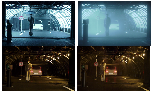
Figure 1: Examples of the Cerema AWP dataset. The same pedestrian appears roughly at the same place in different weather and light conditions.
