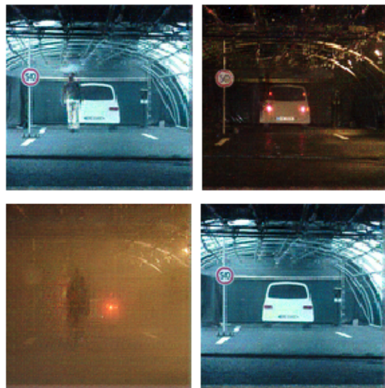
Figure 5: Examples of generated images using a conditional DCGAN-like architecture on images of size 128 \times 128 . The weather is uniform on each image but the pedestrian is not well generated or ignored.
